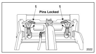
Figure 3-19 Attachment Locks in Locked Position
